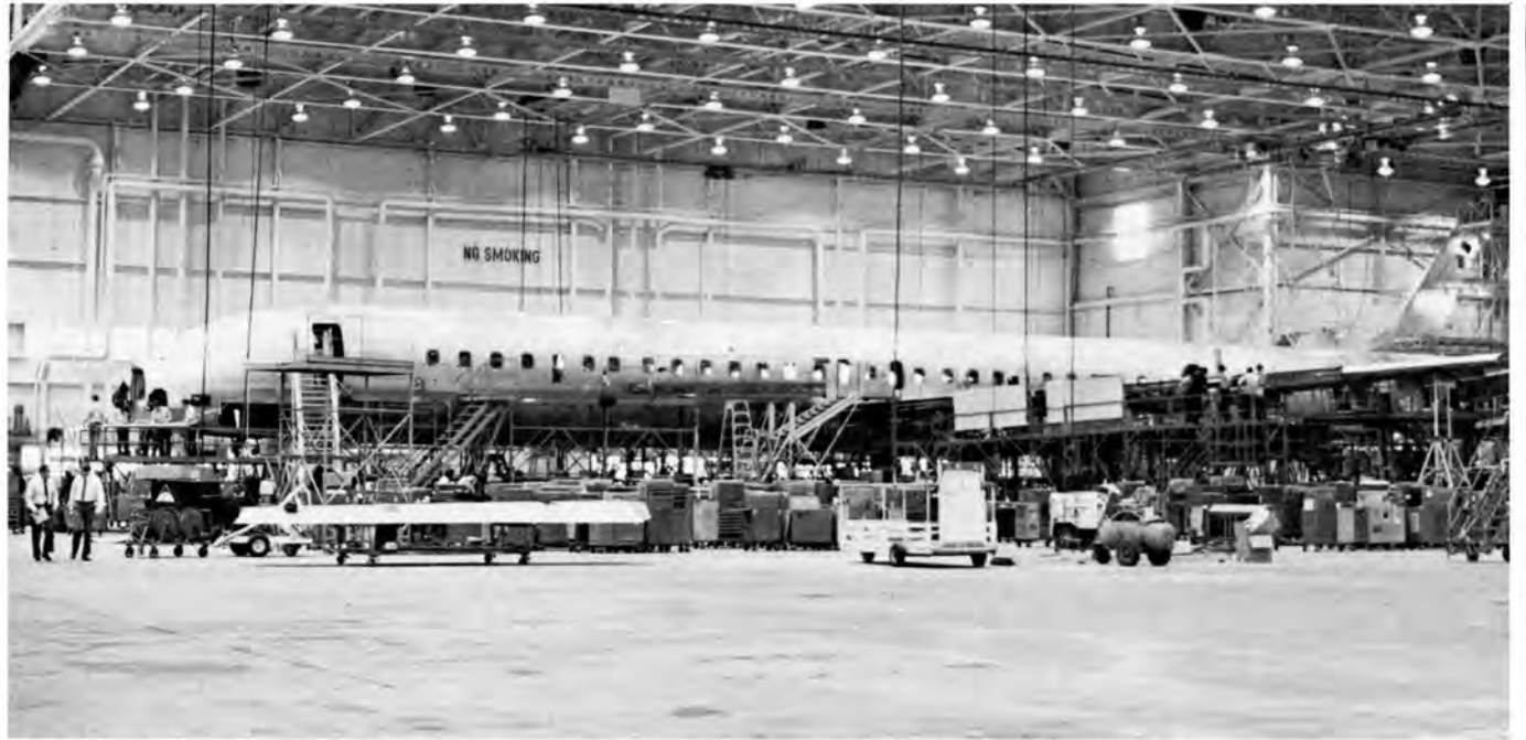
MODIFICATION OF THE FIRST DC-8 at Delta's Technical Operations Center in Atlanta began on February 1 and will be completed next month. Hundreds of hours of training were conducted for overhaul and aircraft maintenance personnel as they prepared to modify and maintain the DC-8-71 aircraft. A total of 300 mechanics, electricians and inspectors attended the 20-hour modification training classes and another 200 have attended the 20-hour maintenance classes.
