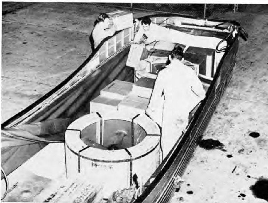
The speedpak, a prominent feature on the Constellation, were capable of hauling 8,000 pounds per trip. They were operated between Chicago and Caracas via St. Louis, Memphis, New Orleans, Havana and Kingston.
