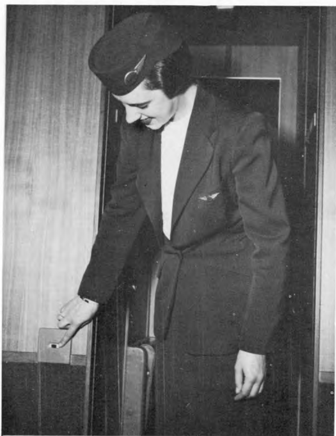
ALTERNATE SWITCH—CABIN AISLE NIGHT LIGHTS located on bulkhead at forward end of main cabin, Night lights may also be controlled from Stewardess switch panel.
