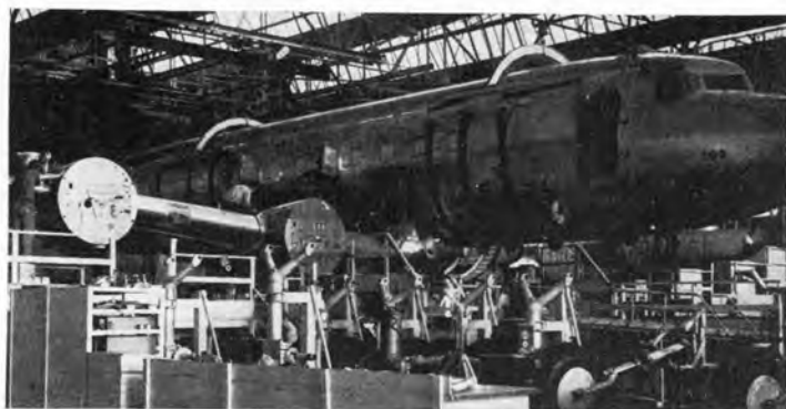
A major step in the assembly is the mating of the wing section and fuselage. From here, the planes roll forward on their own gear.
