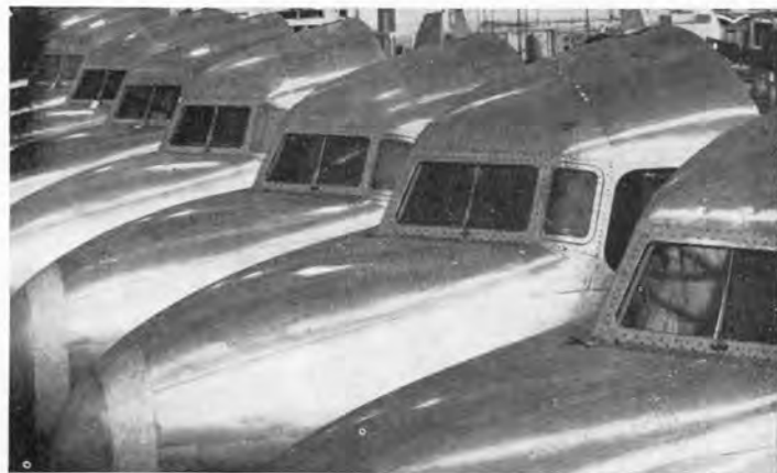
The nose sections, except for internal fittings. They are seen lined up to go on DC-6's, 6A's, 6B's, or DC-7's.
