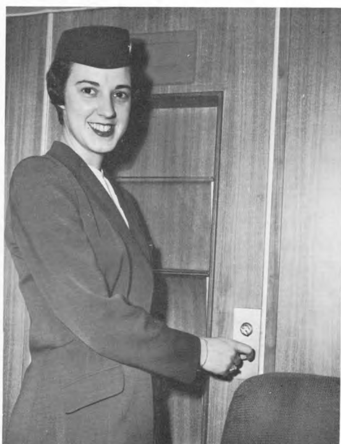
COCKPIT—CABIN DOOR LOCK —opened with cockpit key. (Same key used on CV-340, DC-6 and DC-7.) A spare key is stored in the compartment over the left coatroom.
