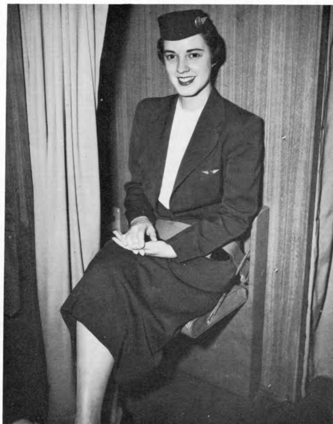
STEWARDESS SEAT—AFT CABIN located in left coatroom. Seat folds against bulkhead when not in use.
