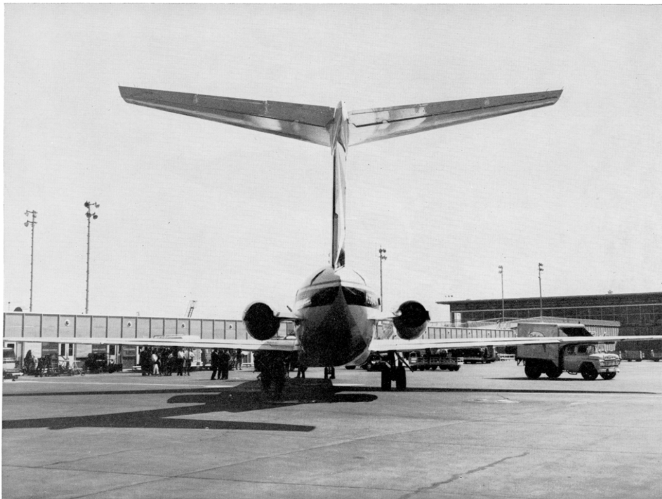
High-level horizontal stabilizer mounted atop the rudder assembly is distinctive DC-9 feature.
